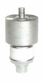
Input of 14 kW is permissible up to 110 MHz. Plentiful reserve emission is available from it's 386 watt filament. The grid structure is rated at 150 watts making this tube an excellent choice for industrial service.
