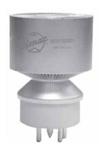
The 3CX1500D7 is a compact, high-mu triode with an anode dissipation rate of 1500 watts. This power grid tube features high gain and operates with zero bias in Class AB<sub>2</sub> as a linear amplifier; or with simple cathode bias, it provides good efficiency in Class B and Class C. A single 3CX1500D7 will replace two 3-500Z's in many applications.
