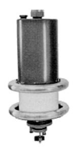
The 4CPW300,000A/9008 is a water-cooled power tetrode intended for use as a pulse modulator or in pulse regulator service. The tube is rated for 100 kVdc holdoff in a protective atmosphere, with a 90 amperes pulse cathode current rating during conduction and a 300 kW anode dissipation rating (average during pulse). Peak anode current capability in excess of 150 amperes for short pulse operation is practical.
