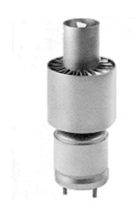
The 3CX1000A3 is a forced-air cooled, ceramic/metal medium-mu triode designed primarily for use in industrial RF heating services. Input of 9 kW is permissible up to 75 MHz. Plentiful reserve emission is available from its 233 watt filament. The grid structure is rated at 75 watts making this tube an excellent choice for industrial service.
