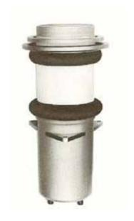
The 3CW150,000H3 is a water-cooled, ceramic/metal, medium-mu power triode designed primarily for use in industrial RF heating services. Its water-cooled anode is conservatively rated at 150 kW of plate dissipation with low water flow and pressure drop. Input of 320 kW is permissible up to 30 MHz. Plentiful reserve emission is available from its 310 watt filament. The grid structure is rated at 1500 watts making this tube an excellent choice for industrial service.
