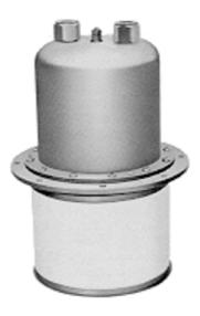
The 4CW150,000E is intended for use as a Class C RF amplifier or oscillator, Class AB push-pull AF amplifier or modulator as well as a plate and screen-modulated Class C RF amplifier. In pulse modulator service, it can deliver a peak output of 4 megawatts. The tube is characterized by low input and feedback capacitances and low internal lead inductances.
