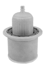
The 4CW100,000E is ideal for use as a Class C RF amplifier or oscillator, a Class AB RF linear amplifier, or a Class AB push-pull AF amplifier or modulator as well as a plate and screen-modulated Class C RF amplifier. In pulse modulator service, it can deliver a peak output of 4 megawatts. The tube is characterized by low input and feedback capacitances and low internal lead inductances.
