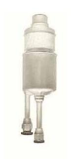
The 3CW5000A7 is a water-cooled high-mu triode intended for use as an RF amplifier in industrial applications where water cooling is preferred over air cooling. This tube is a water-cooled version of the 3CX3000A7.
