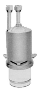
The 3CW40,000A5 is a medium-mu power triode designed primarily for use as an RF power amplifier. Input of 100 kW is permissibleup to 90 MHz. Plentiful reserve emission is available from its 1500 watt filament. The grid structure is rated at 1000 watts dissipation. The electrical characteristics of the 3CW40,000A5 closely match those of the Siemans RS2021W and it is, therefore, ideal as a retrofit.
