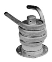
The 3CW2500C7/YU-157 is a rugged coaxial base power triode designed for use as a cathode driven Class AB<sub>2</sub> or Class C amplifier. It is recommended for VHF or UHF service as a linear amplifier, power amplifier or pulse amplifier. Linearity and power gain are both excellent due to the low ratio of grid-to-plate current and the relatively high amplification factor. This tube is a water-cooled version of the 8939/3CX1500C7.
