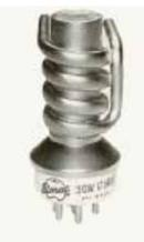
The 3CW1750A7 is a water-cooled high-mu triode intended for use as an RF amplifier in industrial applications where water cooling is preferred over air cooling. This tube is a water-cooled version of the 3CX1200A7.
