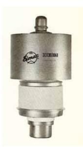
The 3CX3000A1/8238 low-mu power triode is forced-air cooled and is intended for use as an audio amplifier or modulator. Available high plate current under Class AB<sub>1</sub> operating conditions permits high power gain with a minimum of distortion. The tube is coaxial in construction.
