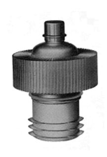
The 3CX1000A7/8283 high mu triode is intended for Class  $AB_2$  linear amplifier service in either grid-driven or cathode driven configuration. It is recommended for use as a grid-driven push-pull audio amplifier or modulator and as a cathode driven linear amplifier through the VHF-TV bands.
