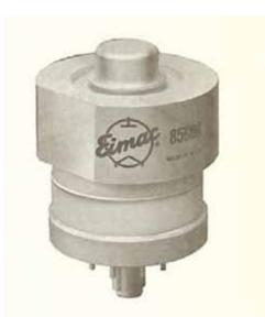
The 8560AS is intended for use as an RF amplifier or oscillator or in audio amplifier or modulation service. It has electrical characteristics similar but not identical to the 4CX250B/7203. The 8560AS is designed for conduction cooling and is nominally rated for 200 watts anode dissipation.
