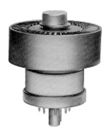
The 4CX600JB is the lower priced version of the highly linear 4CX600J. This type is recommended when operation is to be Class AB, or when extra drive power is available for AB, operation.
