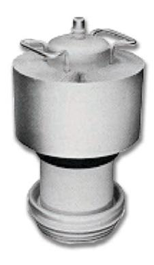
The 4CX35,000/8349 is intended for use at the 50 to 150 kW output power level. It is recommended for use as a Class C RF amplifier or oscillator, a Class AB RF linear amplifier, or a Class AB push-pull AM amplifier or modulator
