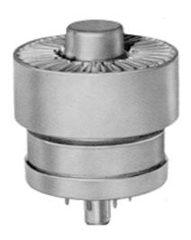
The 4CX250BC/8957 is especially recommended as a premium quality replacement for the 4CX250B/7203 in applications where long life and consistent performance are of prime concern and the closer heater voltage tolerance and increased cathode warm-up time are acceptable.
