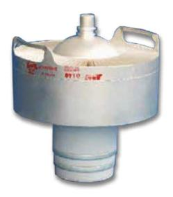
The EIMAC 4CX25,000C is a ceramic/metal power tetrode intended for use as a VHF power amplifier. It features a type of internal mechanical structure which results in high rf operating efficiency. Low rf losses in this structure permit operation at full ratings to 110 MHz.
