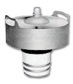
The 4CX20,000B is intended for use as a Class C RF power amplifier in AM broadcast service, for use as a push-pull audio amplifier or modulator, or as a pulse modulator. The anode is rated for 20 kW dissipation and incorporates a highly efficient cooler of new design, which significantly reduces air pressure and flow requirements and produces low acoustical noise.
