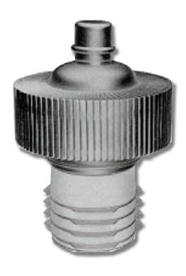
The 4CX1000A/8168 is a low voltage, high current tetrode specifically designed for Class AB1 RF linear amplifier or audio amplifier applications where its high gain and low distortion characteristics may be used to advantage
