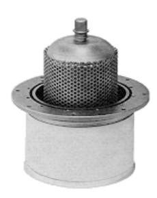
The 4CV50,000E is characterized by low input and feedback capacitances and low internal lead inductances. A rugged thoriated tungsten mesh filament provides adequate emission over long operating life. It is recommended for use as a Class C RF amplifier or oscillator, a Class AB RF linear amplifier, or a Class AB push-pull AF amplifier or modulator. The 4CV50,000E is also useful as a plate and screen modulated Class C RF amplifier.
