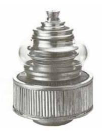
The ML-7003A is a ruggedized shielded-grid triode capable of withstanding severe condisions of shock and vibration while delivering a peak pulse power output of 2.5 MW in switch tube service. The tube is rated for 90 amperes peak pulse cathode current and can hold off 45 kVdc plate voltage.
