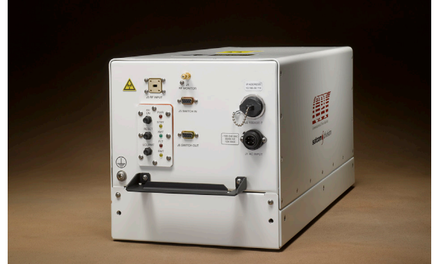
CPI 150 W K-band TWTA, model VZK2791J1.
