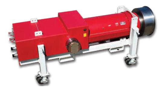
CPI Microwave Power Products (MPP) offers klystrons for particle accelerator applications. The VKL-8301B is a 1300MHz, 10 MW peak, 150kW average, long-pulse Multiple Beam Klystron (MBK) developed for the European X-FEL and International Linear Collider (ILC) projects.
